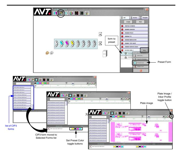
After setting up forms for a job and before starting the job, you can preset the forms with CIP3 data.
